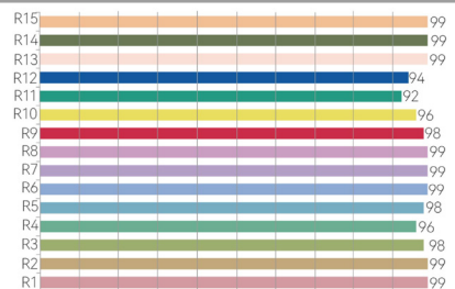
2835 DAYLIGHTCOLOR RENDERING INDEX CCT 6498K Ra=98.4
